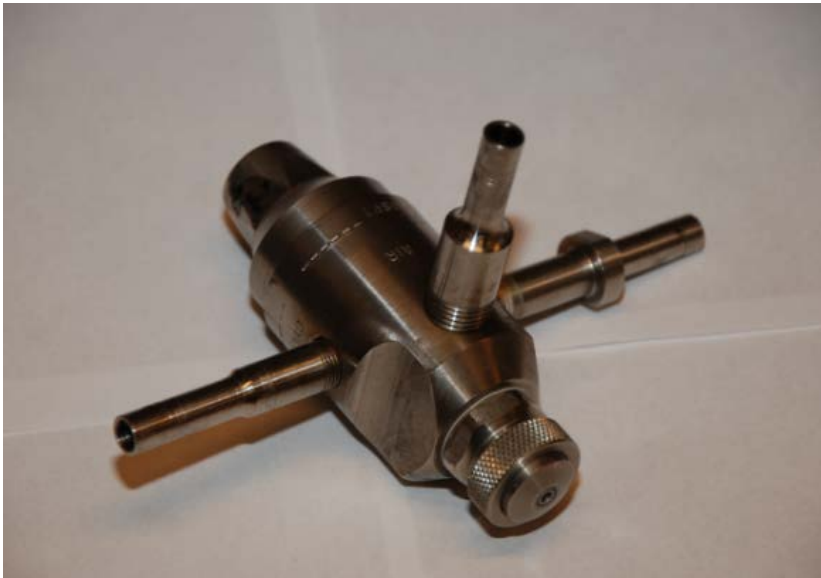
Nozzle using compressed nitrogen gas (1-8 bars)
