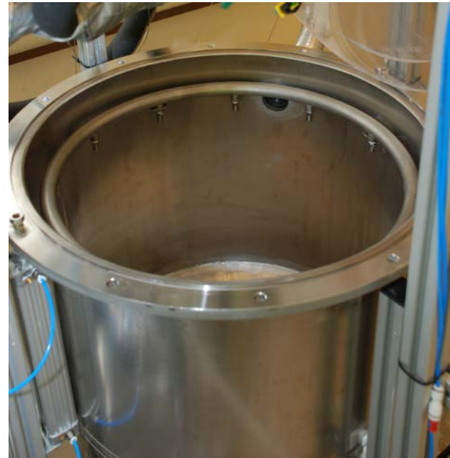
Vessel with n-heptane ESD-PTFE coating
